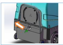
1. Hold the handle of the dustbin buckle and lift it up to loosen the dustbin buckle.
